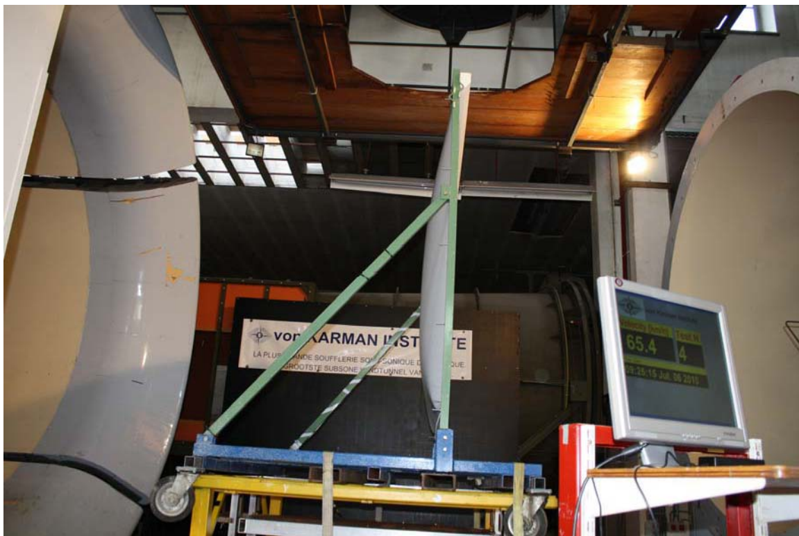
Figure 3: Test 04 Solidscreen® 95 2000 x 2000 mm at 65 km/h 90°
