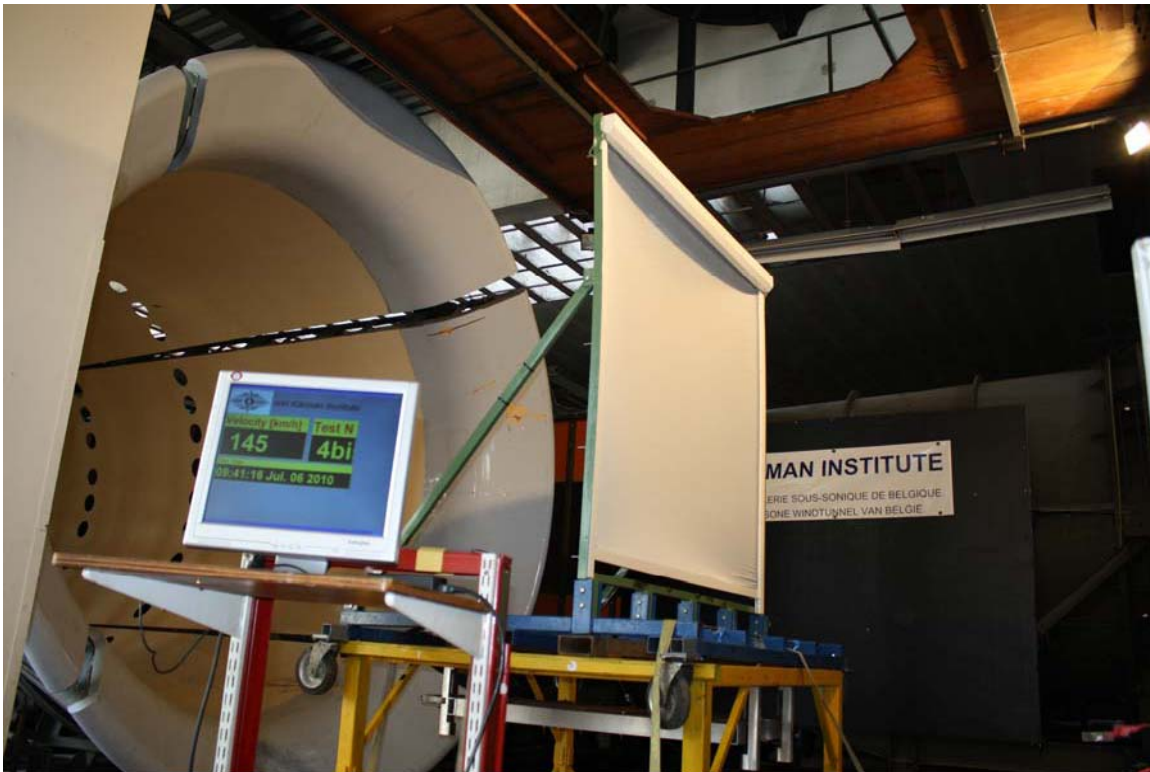
Figure 4: Test 04bis Solidscreen® 95 - 2000 x 2000 mm at 145 km/h 90°
