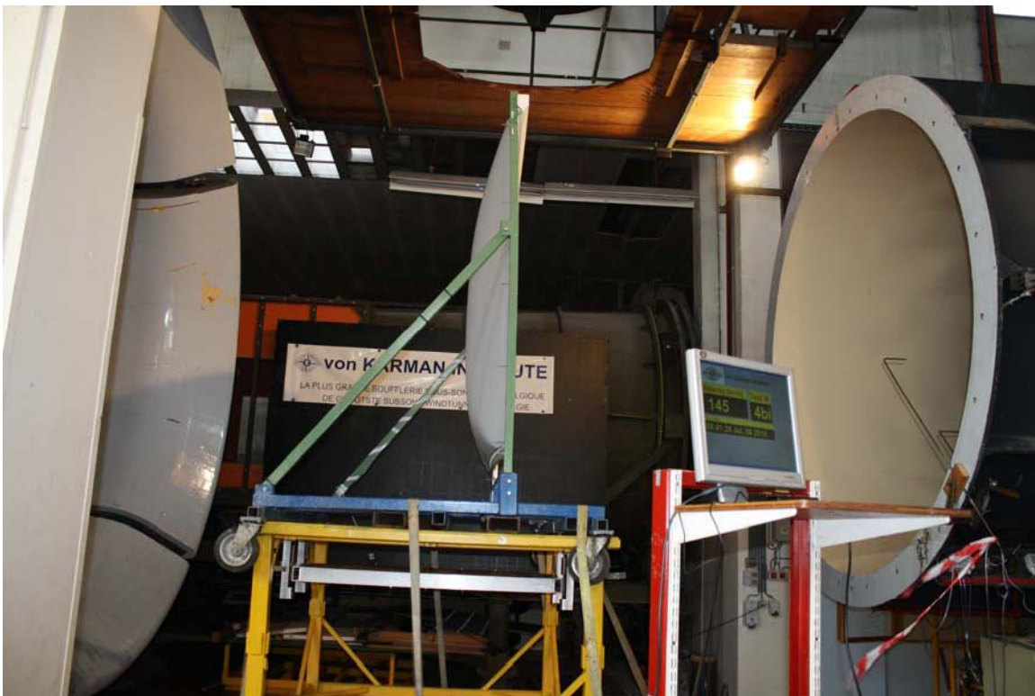
Figure 5: Test 04bis Solidscreen® 95 2000 x 2000 mm at 145 km/h 90°
